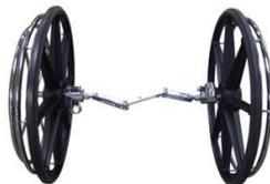
Dual Hand Rim systems consist of 2 hand rims on one side of the chair either Left or Right. The inner hand rim controls the wheel it is attached to. The outer hand rim controls the opposite wheel using linkages instead of a bar to help with folding the chair for storage. Locked with standard wheel locks.
