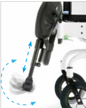
Foot rests , adjustable in height and flexion-extension
